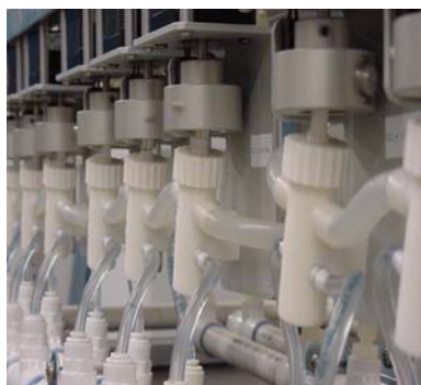
Piston pumps undergoing long-term life testing
